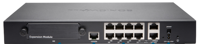
Expansion module Console port 8x1-GbE switch (configurable) X0 LAN port X1 WAN port Secure power
